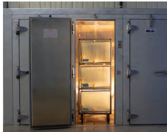
Conditioning of specimens per the "High Humidity Phase" of ASTM E2188.
